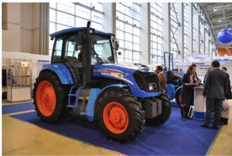
The 85 TX Metan is the bigger of Agromash' two CNG-powered tractors
